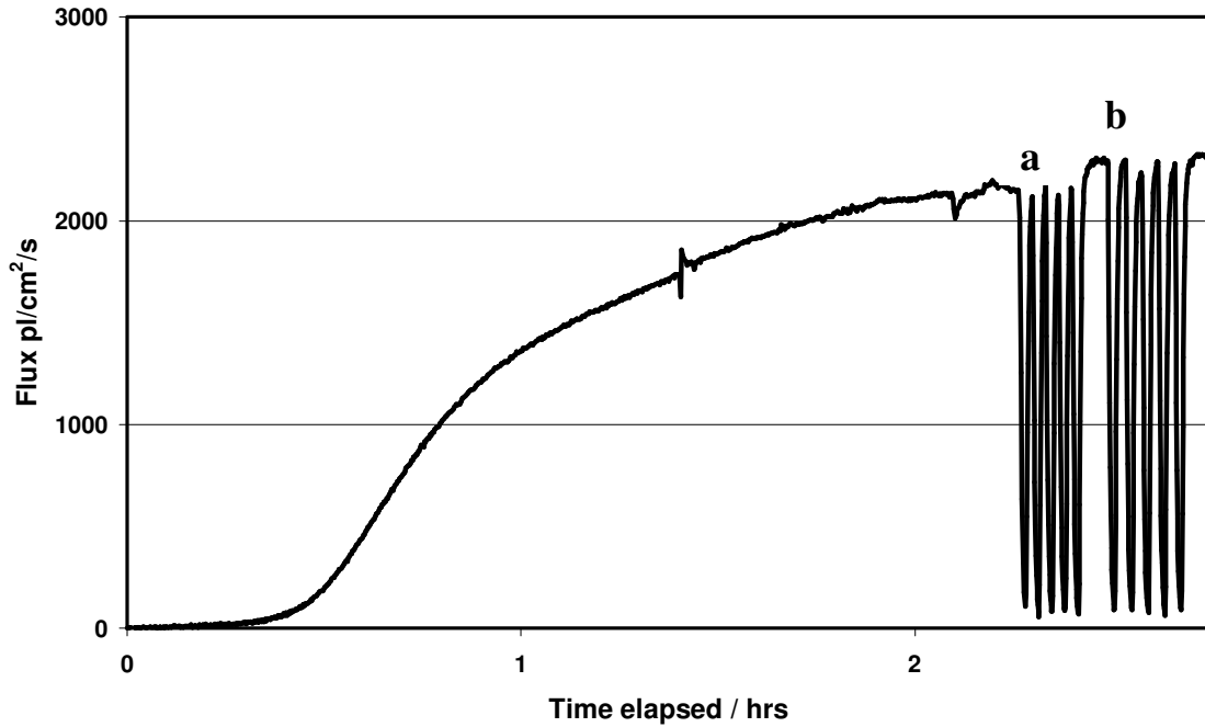
Figure 3. Effect of probe detachment, 80 s manual abrasion of steel exit surface with P120 SiC paper, followed by probe re-attachment on prevailing efflux transient obtained about a week after commencement of the experiment shown in Figure 1 . Flux readings 2000 s subsequent to probe re-attachment are shown by open circles. The anticipated exponential decay profile for efflux without pre-treatment is shown as a broken line.
