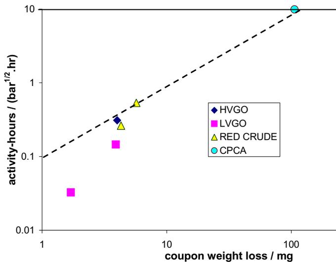
**FIGURE 7 - correlation of corrosion weight loss with hydrogen activity derived from summing over the time of flux profiles shown in Figures 2-4.**
