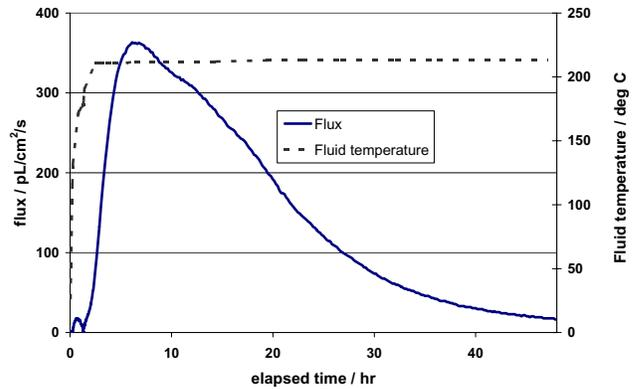
**FIGURE 5 - CPCA in mineral oil, subject to identified fluid temperature excursion. Note extended time scale as compared with Figures 2-4.**
