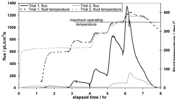
**FIGURE 4 - red crude flux transients, subject to identified fluid temperature excursions**
