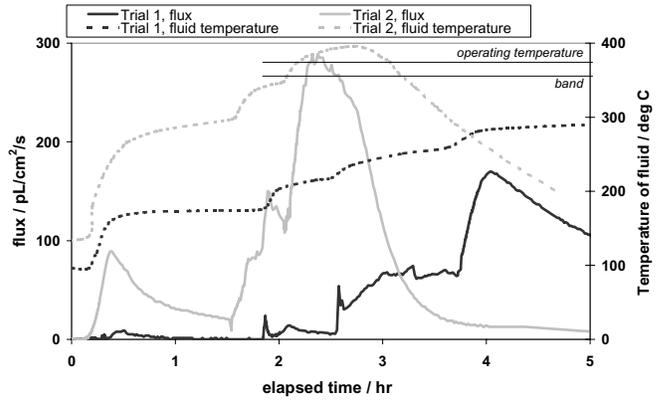
**FIGURE 3 - HVGO flux transients from two trials, subject to identified fluid temperature excursions.**
