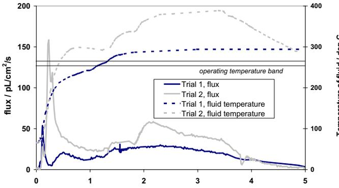
**FIGURE 2 - LVGO flux transients from two trials, subject to indicated temperature excursions.**
